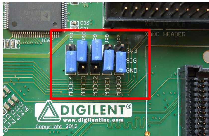
Figure 506: SD Card Boot Settings (ZedBoard)
