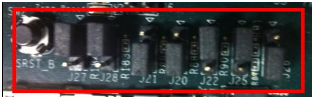
Figure 498: SD Card Boot Settings (ZC702 Board)
