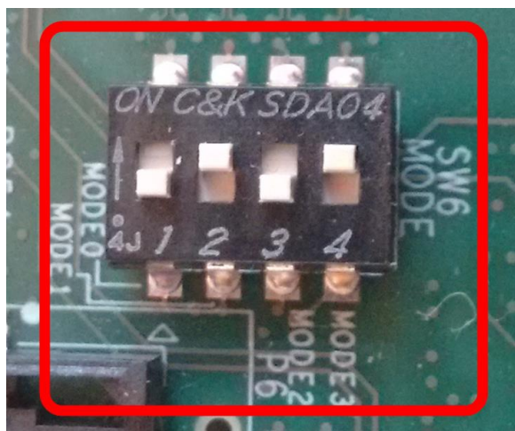
Figure 504: SD Card Boot Settings (ZCU102 Board)
