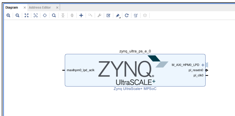
Figure 73: Zynq UltraScale+ MPSoC Block in the Block Diagram
